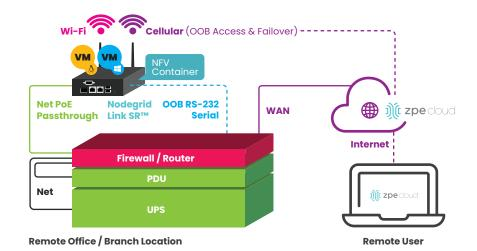
Nodegrid® OS comes standard with the LSR, allowing you to virtualize with guest OS, third-party and custom applications, and Docker, Kubernetes, and LXC containers. Power your LSR via PoE, and connect multiple end devices to deliver critical functionality.
