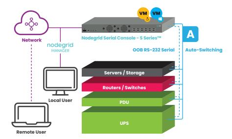
**Doing a serial console refresh? Leave existing cabling intact and simply replace legacy units with the NSC-S.** Nodegrid saves setup and configuration time with legacy serial cable support. Nodegrid S Series cuts cabling costs while granting the freedom to access and manage new deployments based on current pin-outs.
