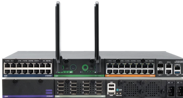
Image: Front/rear views of the Nodegrid Net Services Router with expansion modules for Ethernet, LTE, serial, storage, and USB.
